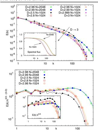
FIG. 1 (color online). (Top) Log-log plot of the mean kinetic energy spectra for different D; in the inset, the mean kinetic energy fluxes. (Bottom) Compensated energy spectra  $E^D(k)k^{5/3-3+D}$  vs the wave number k; in the inset, the compensation is done with the Kolmogorov prediction,  $E^D(k)k^{5/3}$ .
