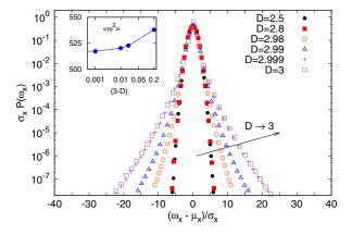
FIG. 2 (color online). Probability density function of the vorticity component  $\omega_x$ , normalized to its standard deviation. Data refer to simulations at resolution N=1024. In the inset, mean square vorticity  $\langle w^2 \rangle$  versus the fractal dimension deficit, 3-D.
