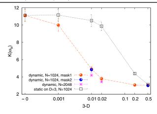
FIG. 3 (color online). Lin-log plot of vorticity kurtosis vs the dimension deficit 3-D. The upper curve is obtained from the application of the *a posteriori* static mask on D=3 velocity field snapshots. The lower curve comes from the Fourier decimated DNS. Data for D=2.99 and D=2.5, with a different realization of the fractal projection, are indistinguishable. Data at resolution N=2048 are also plotted.
