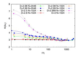
FIG. 4 (color online). Lin-log plot of longitudinal velocity increment kurtosis  $K(\delta v_r)$  vs the scale separation normalized by the Kolmogorov scale,  $r/\eta$ . For all data sets, error bars are within the symbol width.
